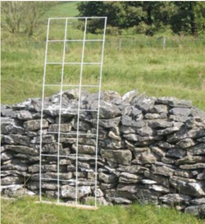
A drawing frame used by CHERT to record each section of wall systematically.
